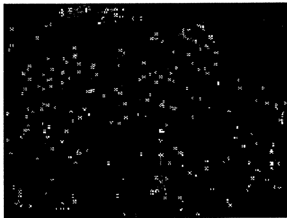
Figure 1. Selective pixel integration selects pixels with a high information content with respect to the variables to be estimated. In this image, the pixels marked in white are informative with respect to pan, tilt and roll of the camera (click on the image to enlarge).
