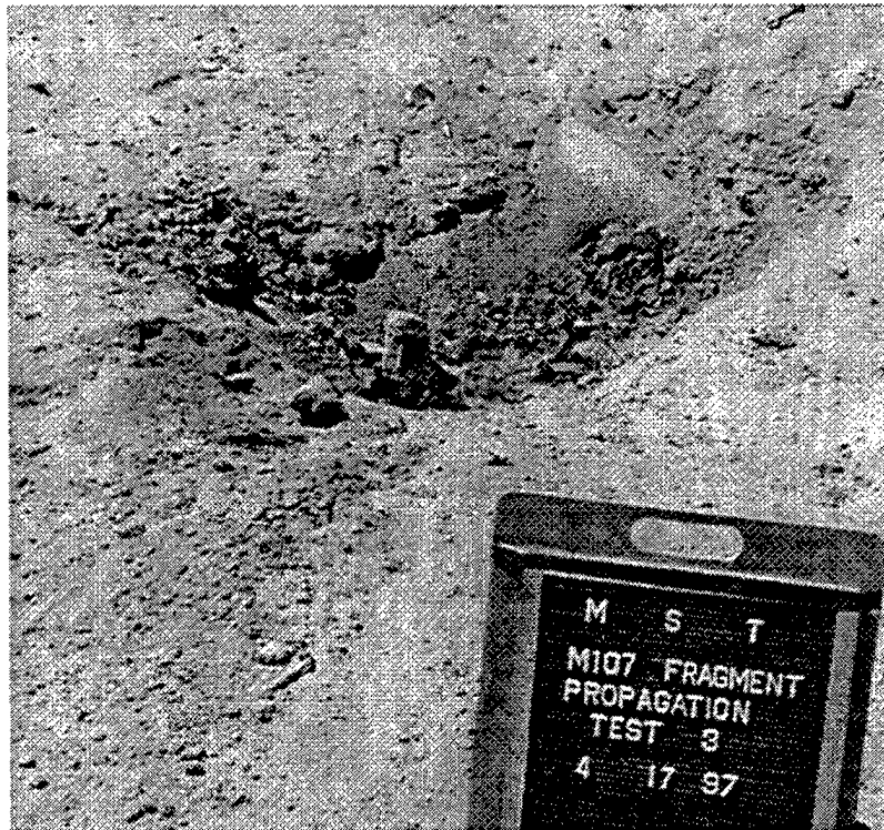
Figure 12. Crater From the East Acceptor Detonation in Test 3.
