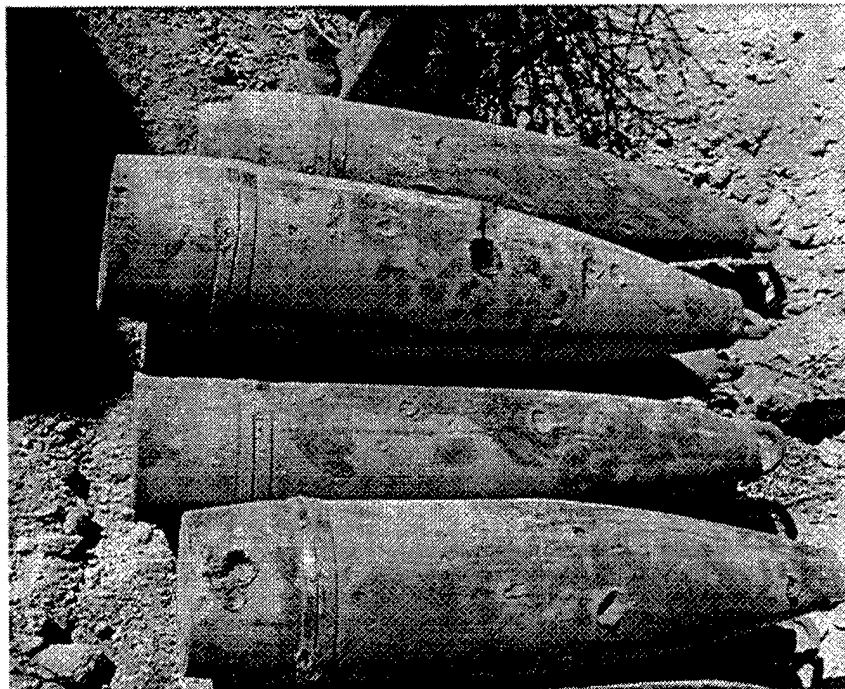
Figure 6. Projectiles From the East Acceptor Stack in Test 1 Showing Impact Craters. Note the Penetrating Impact on the Top Projectile.
