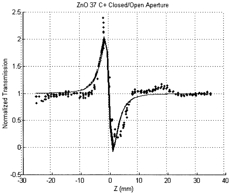
Figure 2. Result of the division of closed and open aperture Z-scans.
