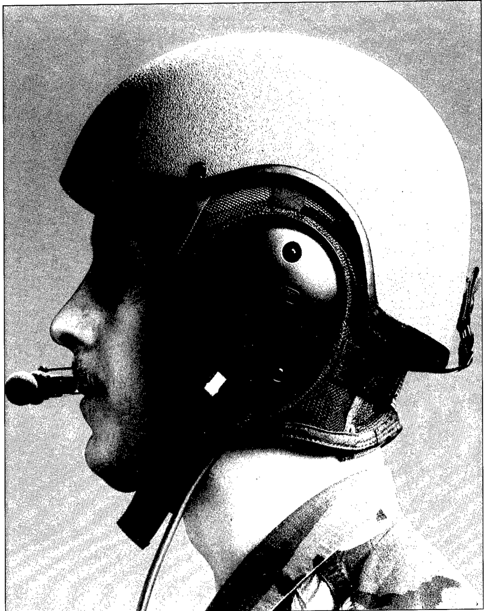
An armored vehicle crewmember wearing a VIS helmet with active noise reduction.
