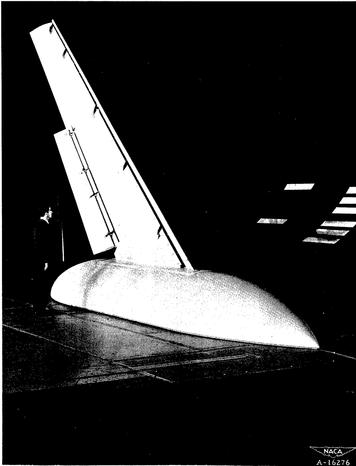
Figure 2.- View of semispan wing-fuselage model installation in the Ames 40- by 80-foot wind tunnel.
