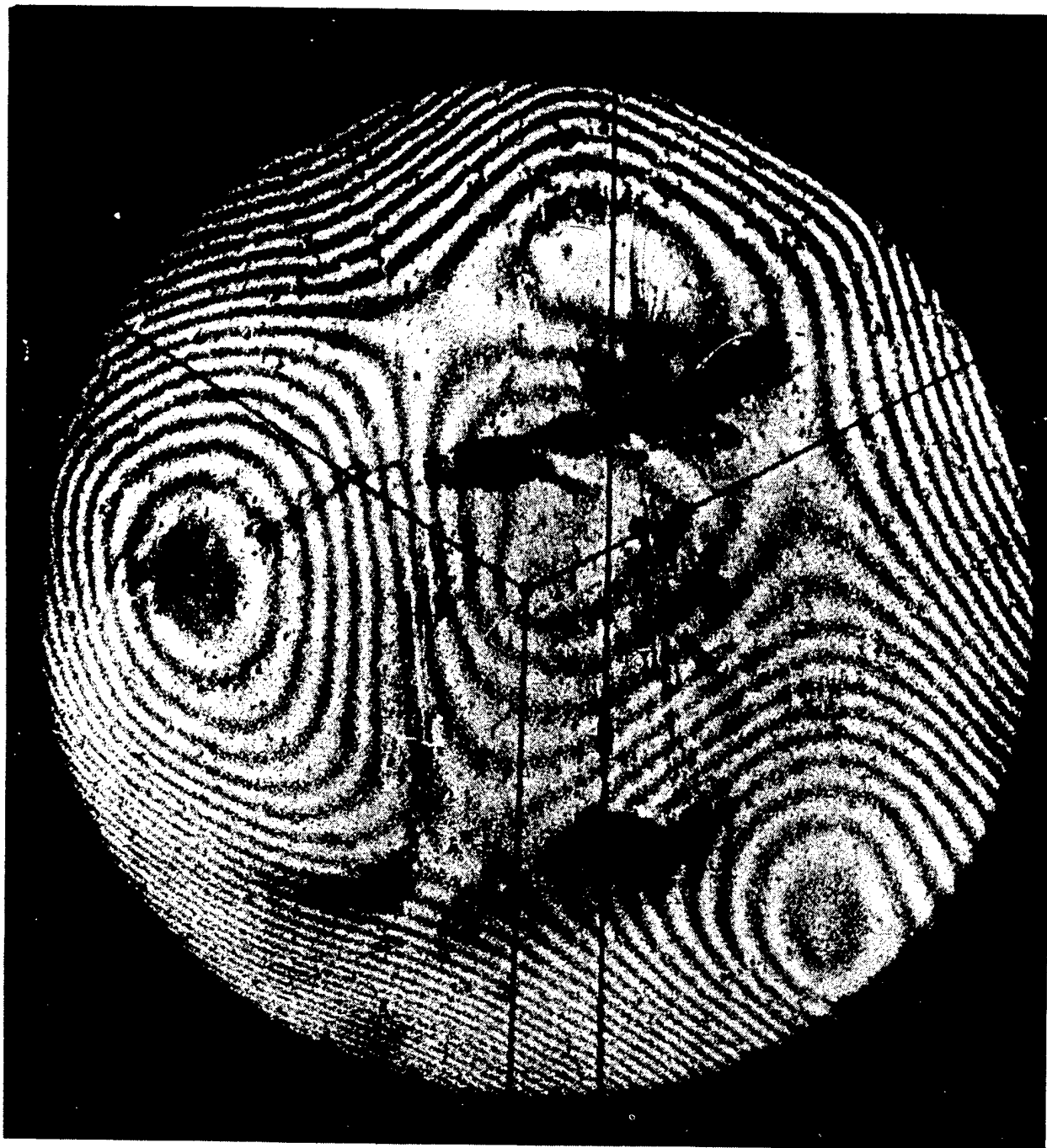
Fig.17 The interference pattern of the surface of a well ground and polished glass plate 36 inches in diameter, 1/4 inches thick, produced by the interference liquid method.
