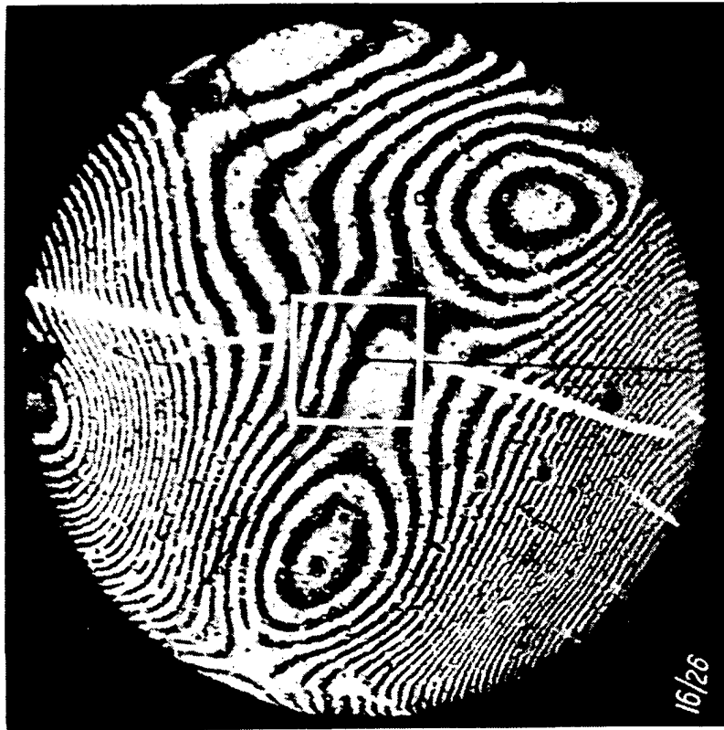
Plate floating in mercury No effect of weight
