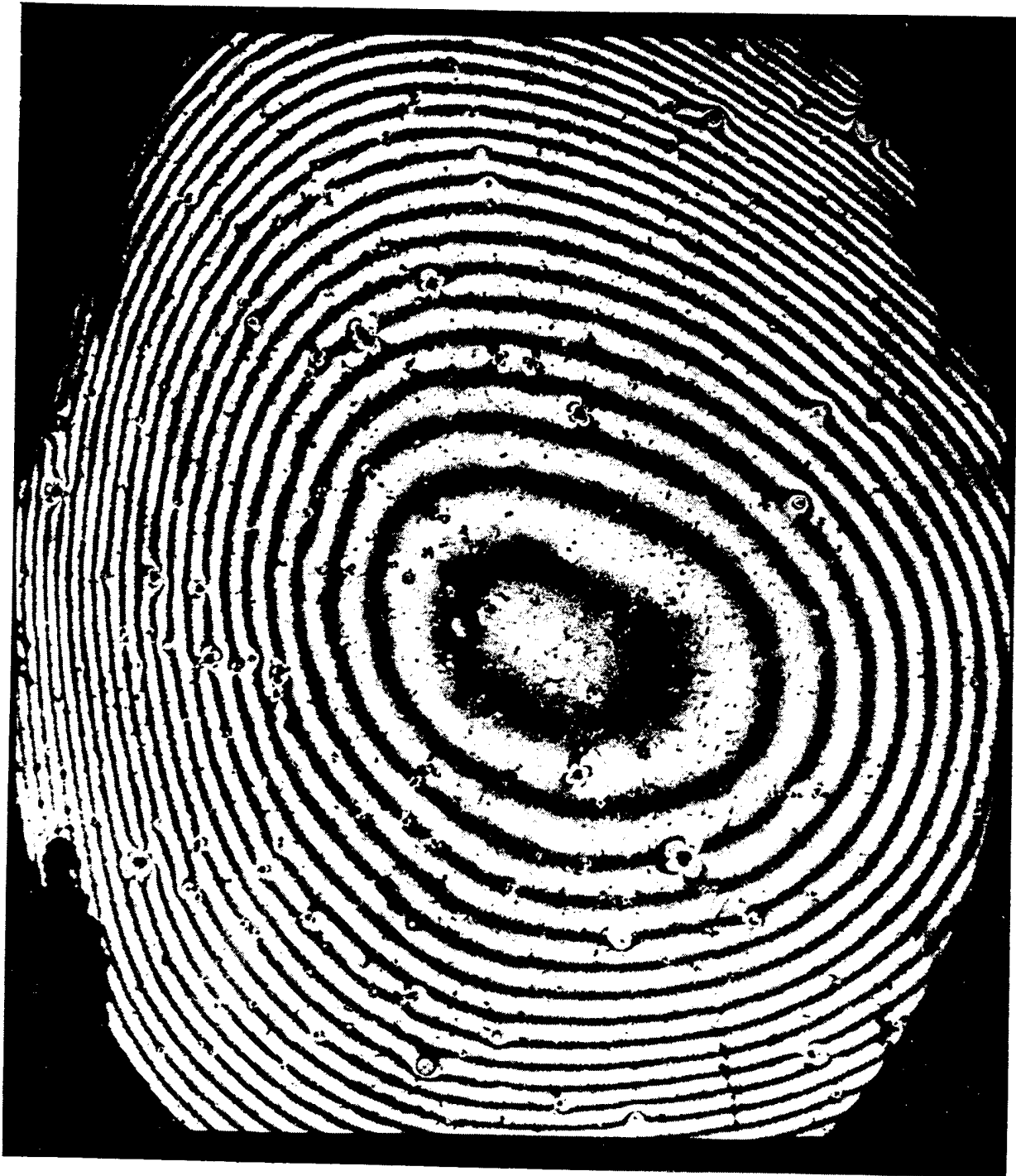
Fig. 14 Interference pattern produced between the surface of a glass plate and the surface of a comparison water layer covering the plate.
