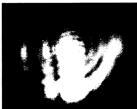
Figure 30. Light from front facet of the distributed Bragg pulse shaper.
