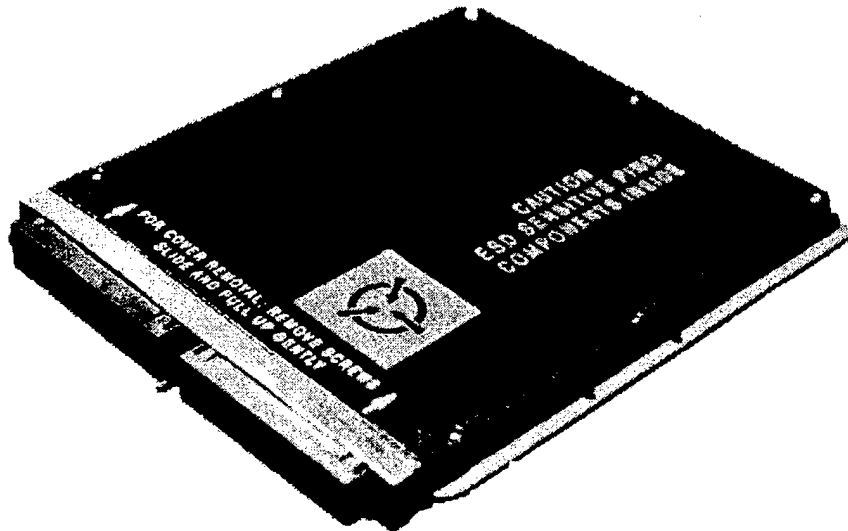
Figure 1. Photograph of typical composite thermal core and covers fabricated by XC Associates
