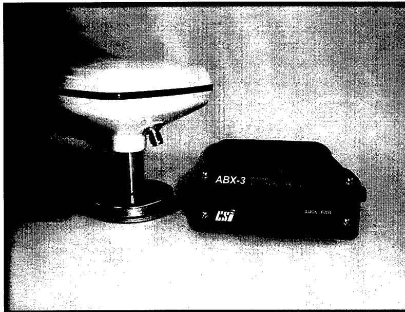
Figure 3.4: Differential Receiver and Beacon [Ref. 5].
