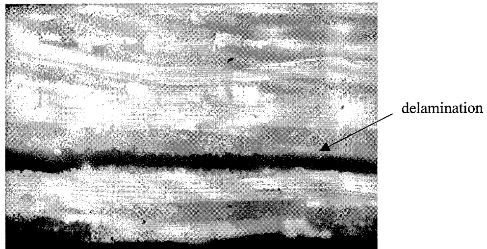
Figure 4-4 Delamination of plies in grip region, 50X
