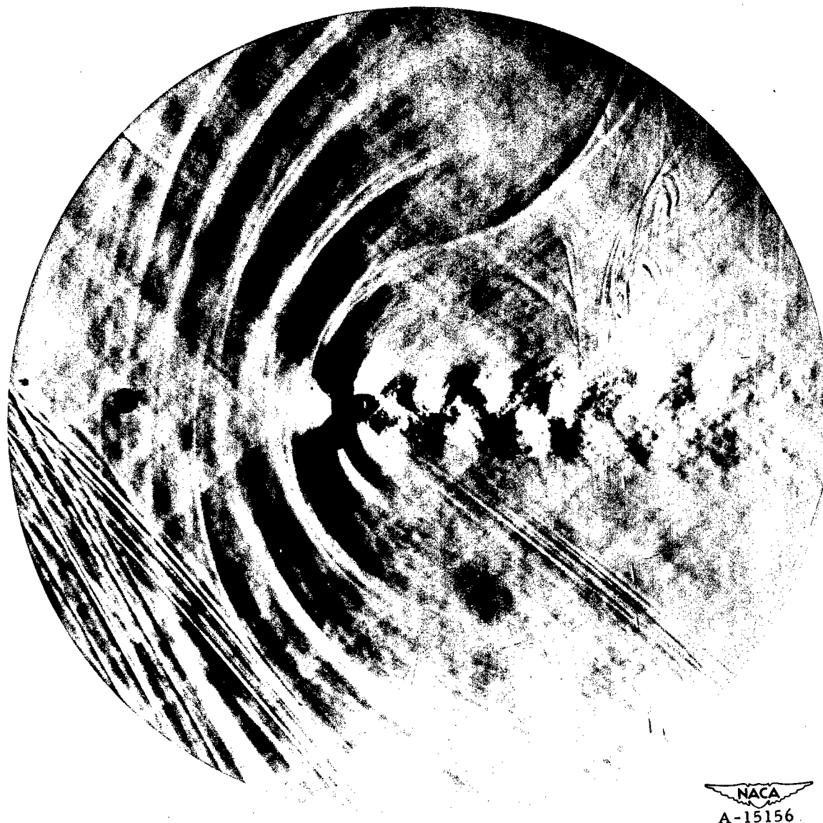
Figure 7.— Vortex discharge from rear of 0.250-inch-diameter cylinder. Discharge frequency, 6250 cycles per second.
