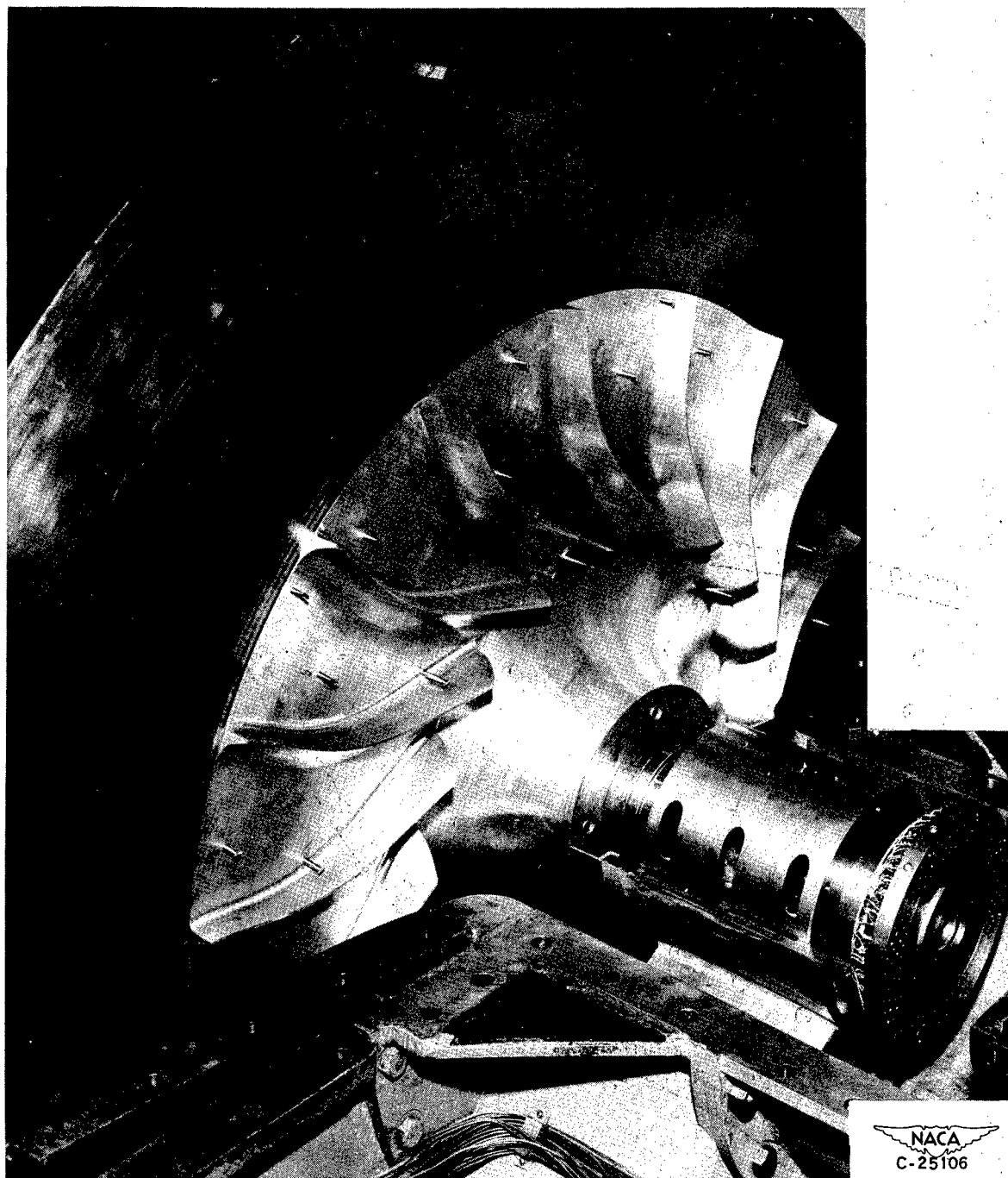
Figure 1. - Radial-inlet impeller used in experimental investigation of flow within rotating passages.
