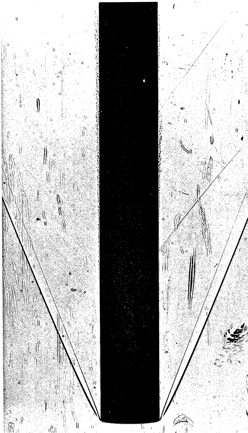
(f) Straight tube; M_\infty = 2.7 ; U_e/\nu = 2.4 \times 10^6/\text{in.} ; H = 10 \mu\text{in.} ; wind tunnel air-off; conical light field; choked internal flow.
