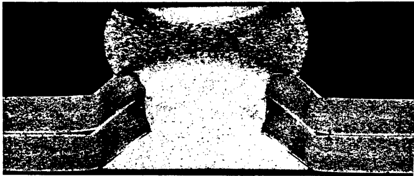
(a) Rivet from joint made by coin dimpling. (Loaded at 125 lb/rivet; lifetime, 2,397,000 cycles.)
