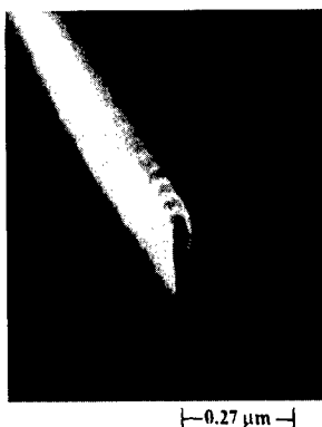
Figure 6. 40 nm line defined in SAL-601 and etched into HgCdTe with \text{CH}_4 + \text{H}_2 . [Ref. 30 with permission.]
