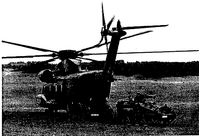
Figure 7 German Army Wiesel I TOW Carriers unload from a CH-53 Helicopter. MAK System Gesellschaft MBH - Light Airtransportable Armoured Systems [WWW page] (The Website for Defence Industries - Army, 2000 [cited 26 March 2000]); available from http://www.army-technonology.com/contractors/armoured/mak/index.html .
