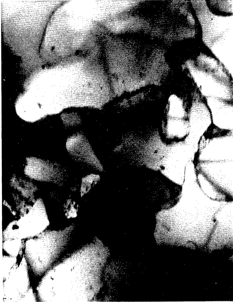
Representative Dislocation Subgranular Structure In Cold Worked 1100-H14 Aluminum 39,000X.
