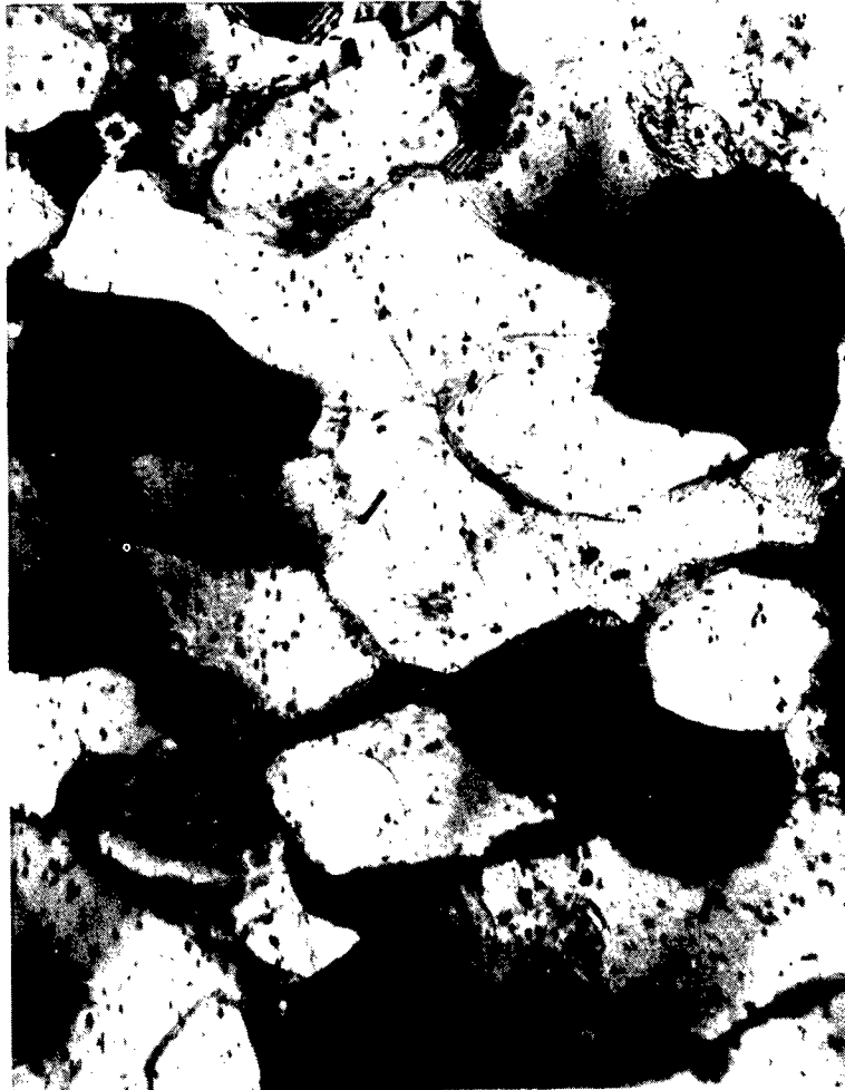
Well Defined Dislocation Subgranular Structure Formed In 1100-H14 Aluminum Fatigued With A Stress Amplitude Of 13,600 psi. Average Subgrain Size Is About 2.0\mu 14,000X.
