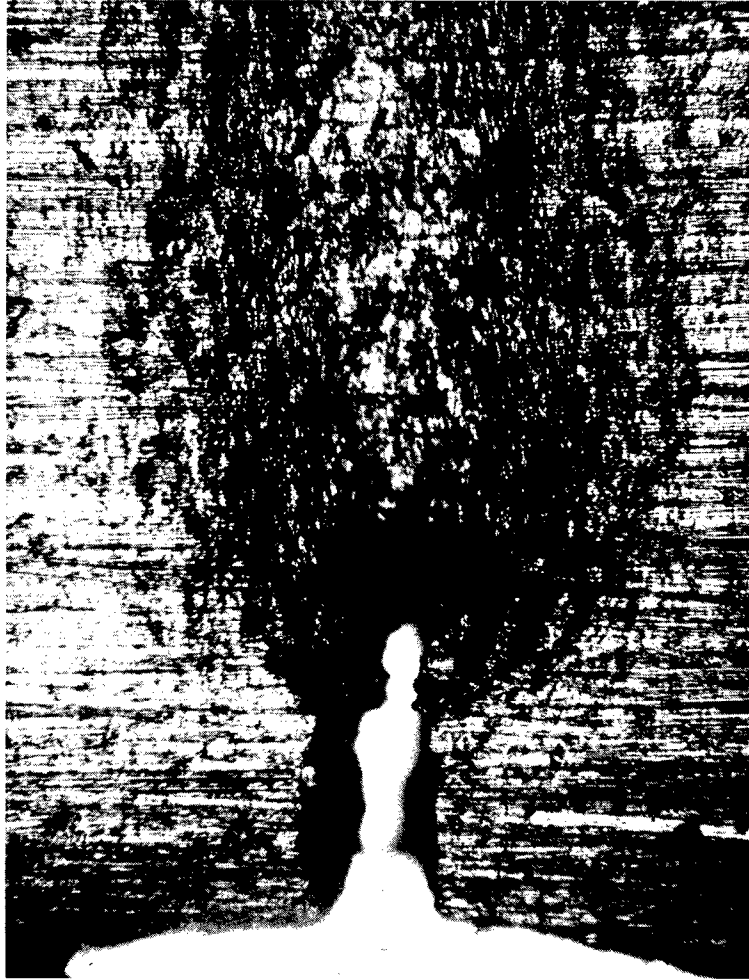
Detail Of Fatigue Crack Originating At Notch And Propagating Into Tensile Specimen Cross-section. Note Plastically Deformed Zone Ahead Of The Crack Front 75X.
