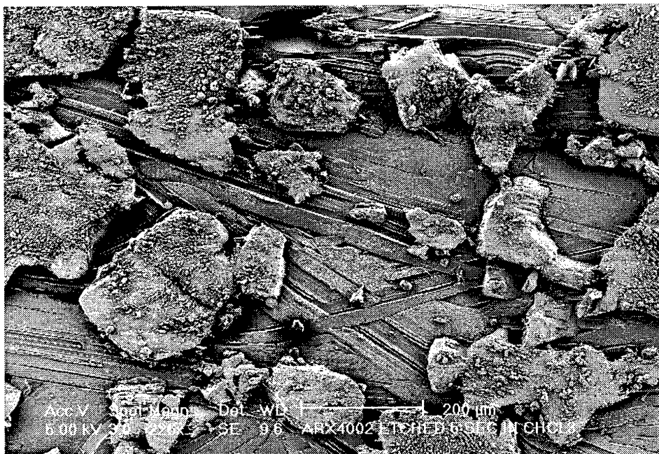
Figure 8. ARX-4002 etched for 5 seconds in chloroform. NTO crystals are standing proud from the TNT grain.
