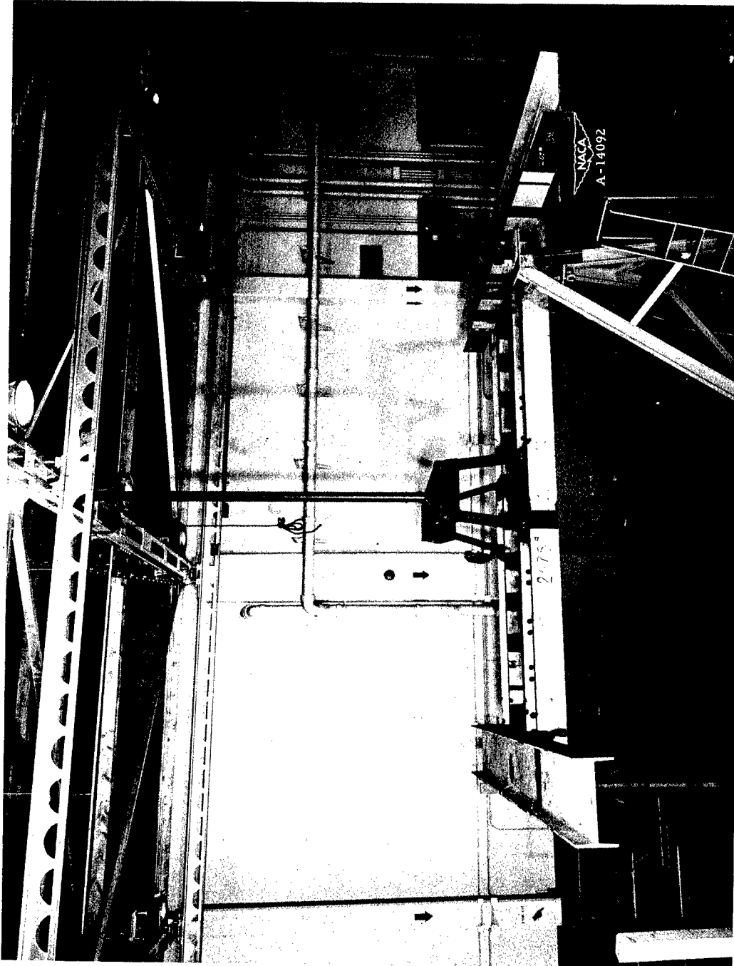
Figure 8.- Torsional-pendulum calibration test frame.
