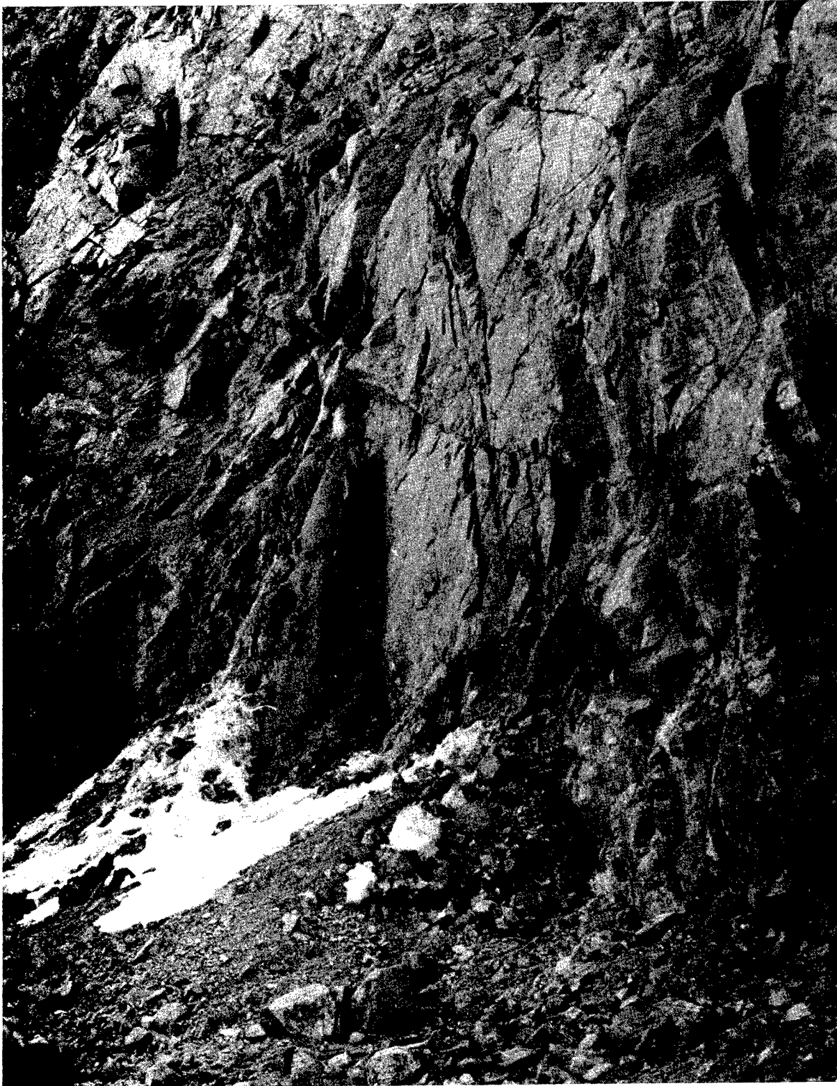
Figure A.37 Kimbley Pit; base of northwestern wall, showing bedrock jointing. (Reproduced by special permission of Kennecott Copper Corporation)
