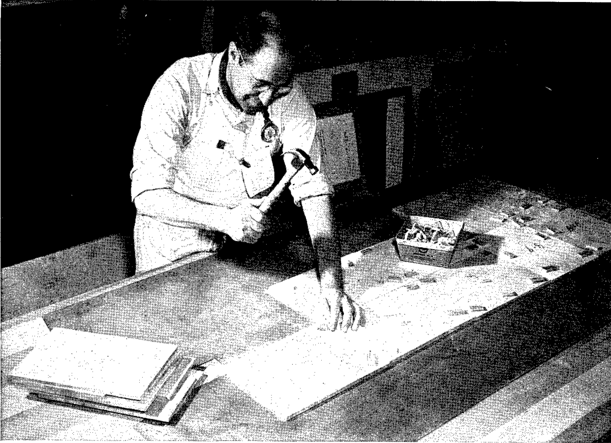
Figure 4-2. Using nail pressure to edge bond end-grain slabs of balsa into larger panels.
