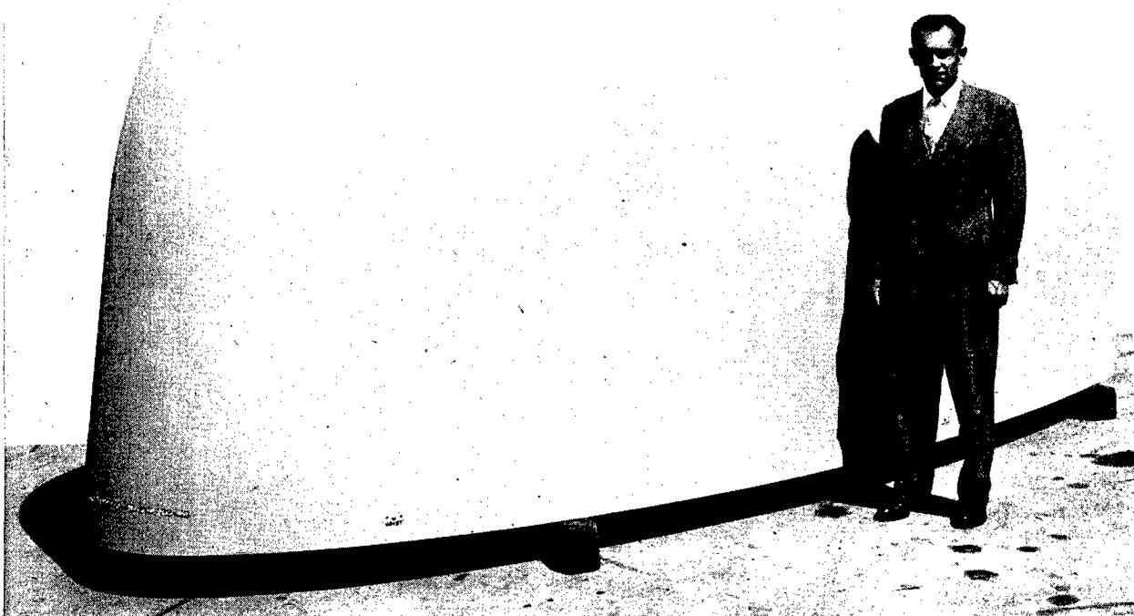
Figure 4-36. Large experimental radome of sandwich construction.
