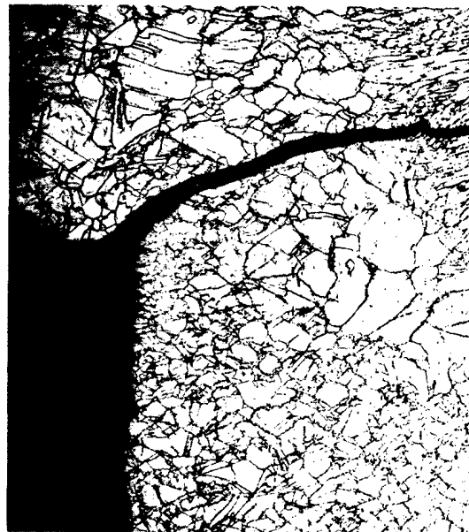
Figure 8 Decarburized zone of inside edge of 3-inch Sch. 40 Type 316 ss pipe after 15,000 hours service at about 1400°F.
