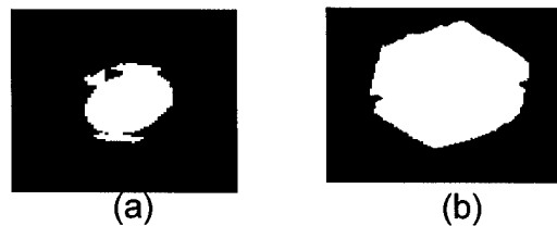
Fig 5: Polaroid prints of the output from the monolithic optic. The source to lens distances in the two cases are 15 mm (a) and 34 mm (b). A copper target with 16 kV tube voltage was used.
