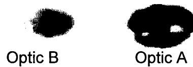
Fig 19: Output images from optic A (22 cm long) and optic B (10 cm long). The defect is seen to be localized to optic A.
