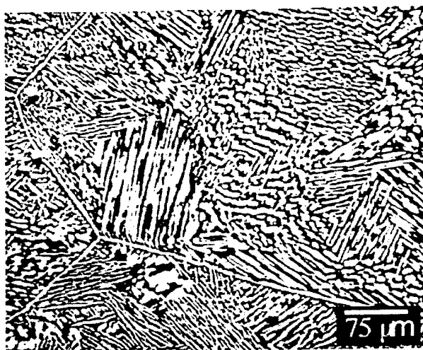
Figure 8.2 BSE-image of the cast microstructure of alloy 10.
