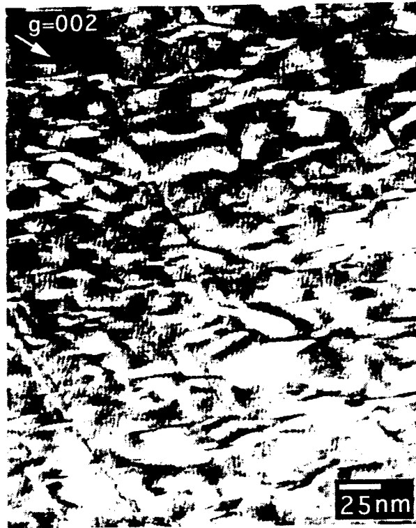
Figure 5.15 Strain induced effects observed under g=002 two-beam conditions within 700^{\circ}\text{C} material.
