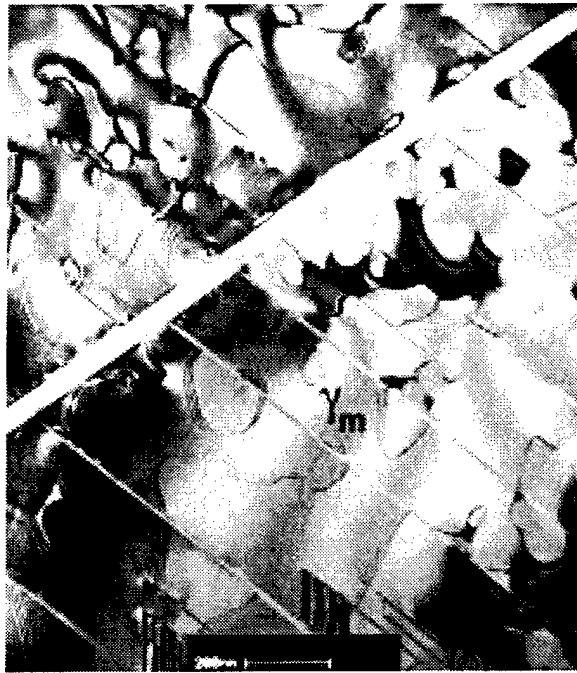
Figure 18. BF TEM micrograph showing the massive \gamma_M phase/microconstituent in the 47-2-2-1 alloy heat treated according to 1370°C/10min. \rightarrow SPQ 1053°C/5sec/WQ.
