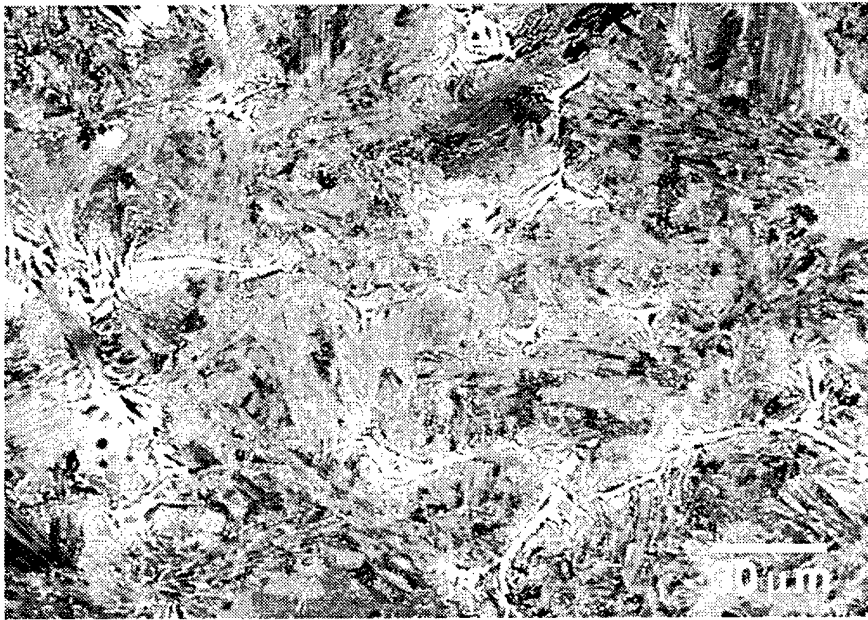
Figure 17. Backscattered electron micrographs of the 47-2-2-1 alloy: (a) \gamma_M + \gamma_F + \gamma_C + \gamma_L + \beta , 1370^\circ\text{C}/10\text{min.} \rightarrow \text{SPQ } 1053^\circ\text{C}/5\text{sec}/\text{WQ} , and (b) \gamma_M + \gamma_F + \gamma_C + \beta , 1370^\circ\text{C}/10\text{min.} \rightarrow \text{SPQ } 1053^\circ\text{C}/300\text{sec}/\text{WQ} . The gray background is a mixture of \gamma_M, \gamma_F, \gamma_L . \beta -phase is imaged light, \gamma_C + \beta appear as the discontinuously growing product from near the grain boundary \beta films into the grain interior.
