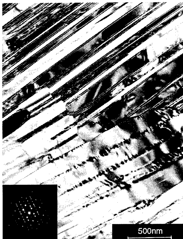
Figure 24. TEM Bright-field micrograph of feathery gamma ( \gamma_p ) microconstituent in 47-2-2-1 alloy. Lamellae viewed edge-on for colony in lower left ( \langle 101 \rangle diffraction pattern), other colonies show small misorientations.
