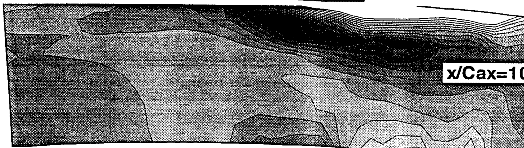
Figure 6.54 axial direction vorticity development (black for anti-clockwise, white for clockwise)
