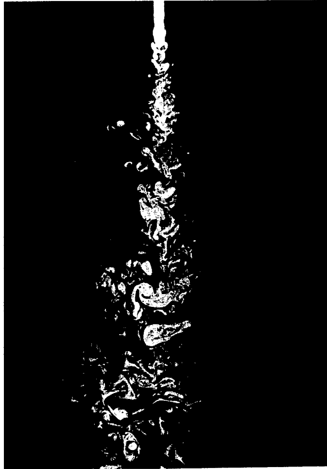
Fig.4. Concentration of a turbulent round jet into water at Reynolds number 2.300, measured by laser induced fluorescence; the cut is along a plane including the axis of a symmetry of the jet. (Reproduced with permission from Dimotakis, Miake-Lye, and Papantonionu (1983).)
