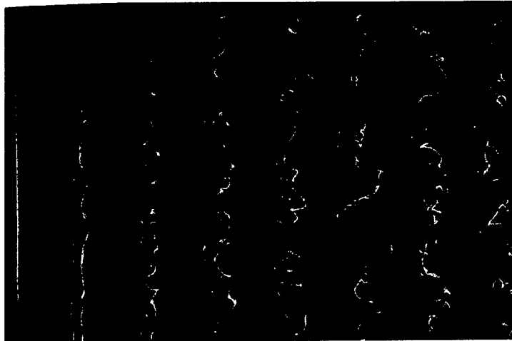
Fig.2. Growth of a “material line” composed of small hydrogen bubbles produced by a platinum wire stretched across an decaying turbulent flow behind a grid placed at the extreme left. The Reynolds number based on the wire diameter is 1.360. (Reproduced with permission from Corrsin and Karweit (1969).)
