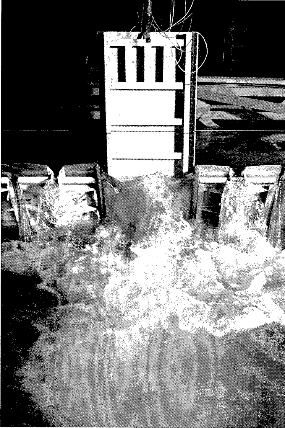
Figure 10. View from the catwalk, looking upstream at the blank at el 287 and an angle of 90 deg. Headwater 301, Tailwater 294; 7-ft differential
