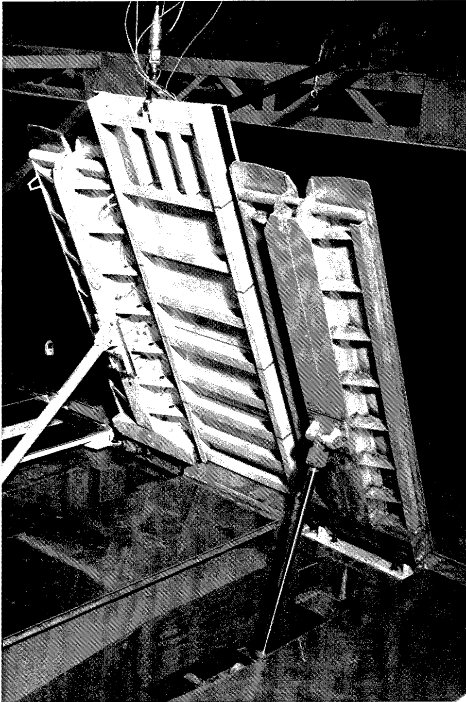
Figure 5. View from the walk, looking upstream at the blank seated on wicket gate #5 at an angle of 65 deg. Dry bed photograph
