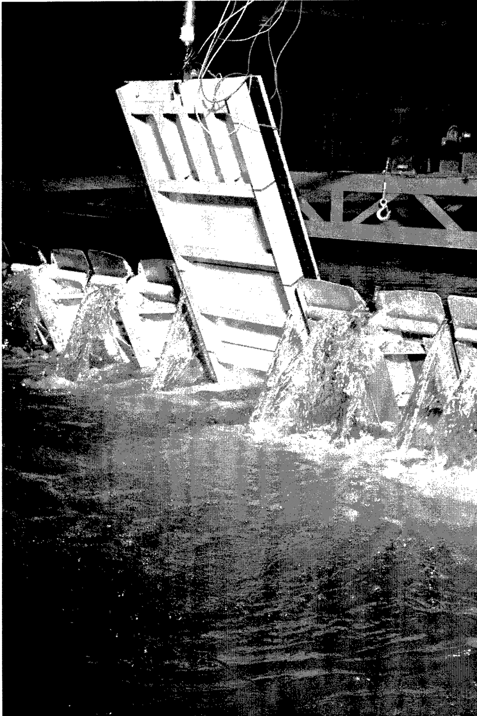
Figure 11. View from the walk, looking upstream at the blank at el 287 and an angle of 65 deg. Headwater 301, Tailwater 294; 7-ft differential
