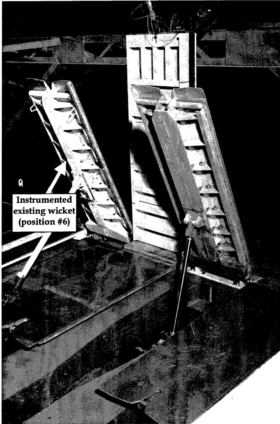
Figure 3. View from the walk, looking upstream at the blank seated on wicket gate #5 at an angle of 90 deg. Dry bed photograph
