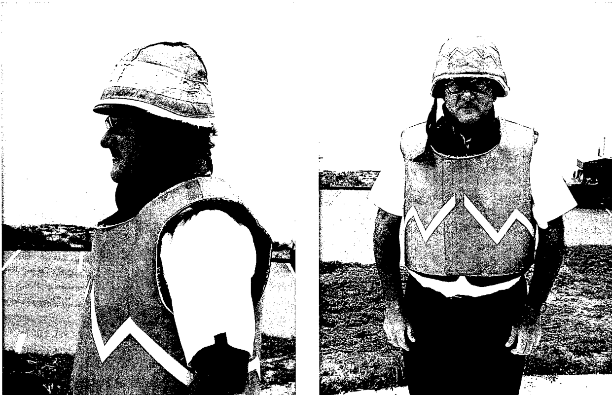
Figure 18. Mark I helmet antenna (side view) and Mark II helmet antenna (front view).
