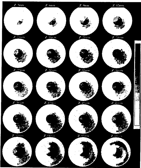
Fig. 5. Images reconstructed from experimental data with the object located at a distance of 15 mm ( z = 45 mm) from the exit plane. The sequence of circles represents images at 3-mm intervals along the cylinder axis.
