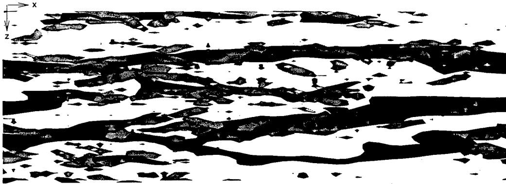
Figure 1. Lifted low-speed streaks (black) illustrated by u' < 0 at y^+ = 20 and streamwise vortices (grey) indicated by the Jeong & Hussain (1995) vortex definition in the region 0 < y^+ < 60 .
