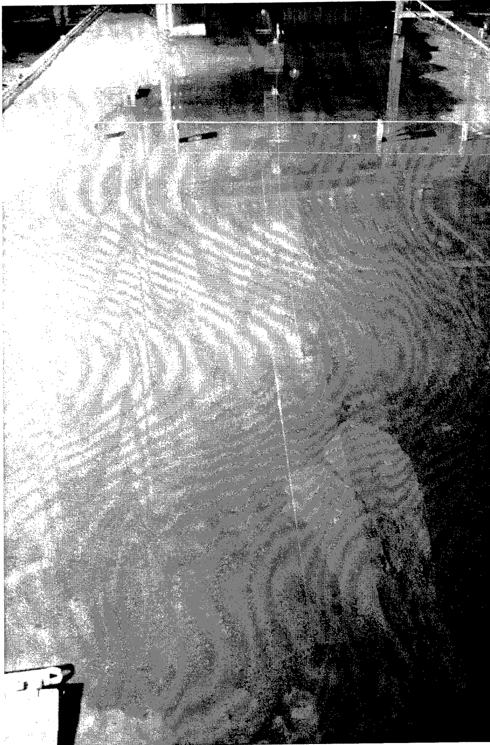
Photo 6. Option 5, discharge 750,000 cfs, looking upstream, showing path of downbound 35-barge tow driving the bend upstream of the bridge
