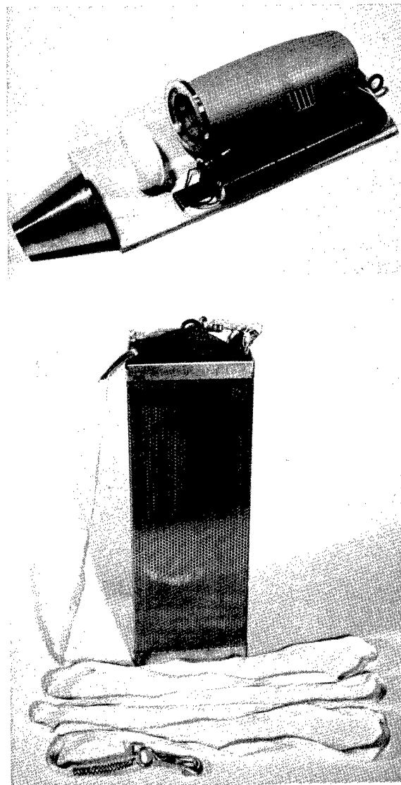
Fig. 28. The parachute-borne integrating air-sampler. Upper, partially disassembled. Lower, assembled.
