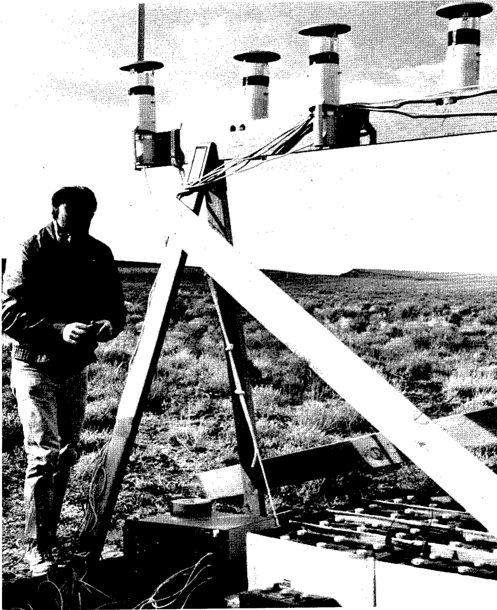
Fig. 3. A nearly completed sequential air-sampling station. The cross-piece holds the sampling heads 7 ft above the ground. A rope is slung under the battery pallet to secure the samples against upset by wind or shock wave.
