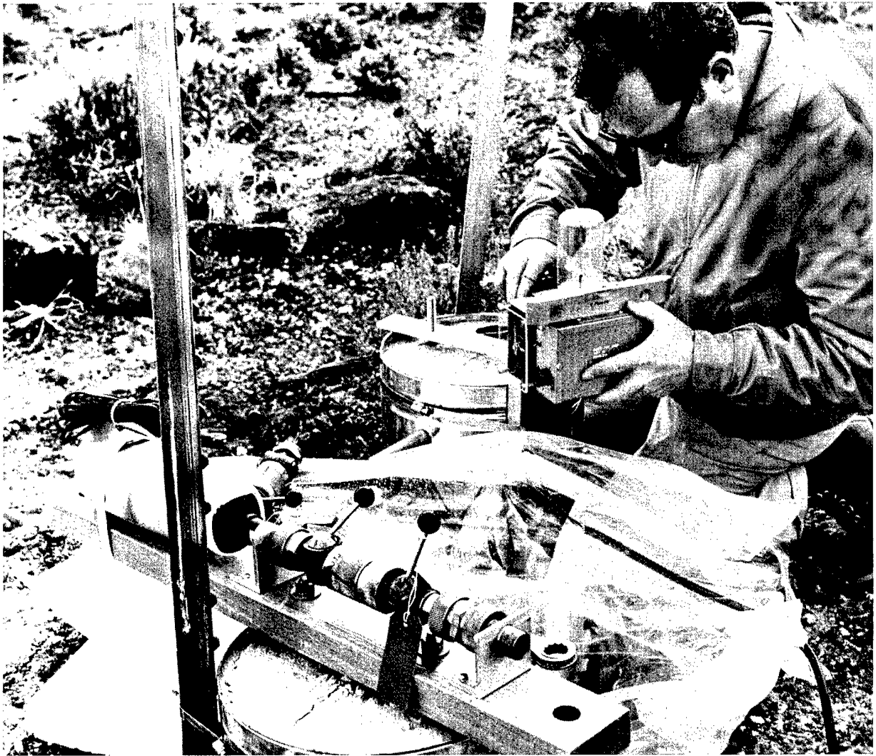
Fig. 33. Installation of a tritium air-sampler in the field.
