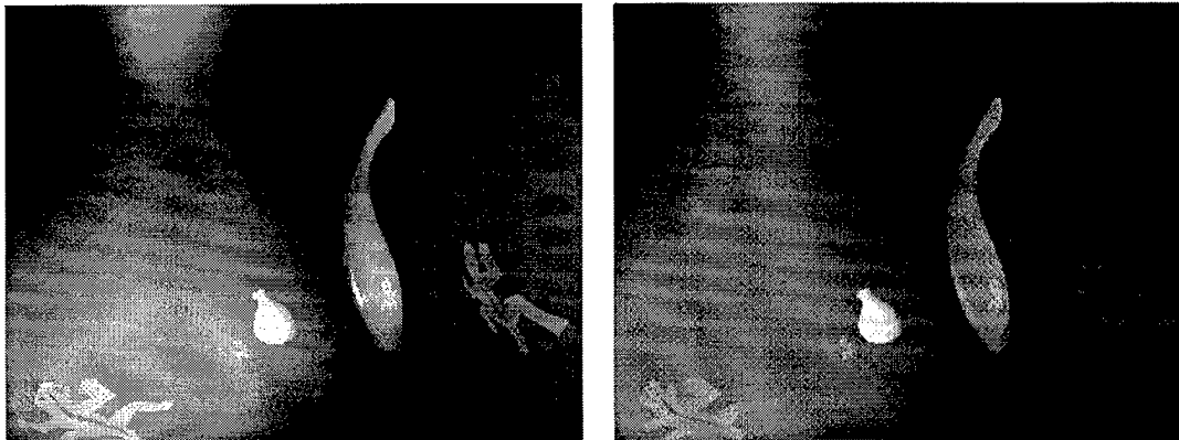
Figure 2: Ray traced scene with multiple reflections (left), and z-buffered scene computed using perturbation of virtual object (right). As the reflected object moves, the z-buffered image can be updated in 0.7 seconds, whereas the ray traced image requires 67 seconds to re-compute.
