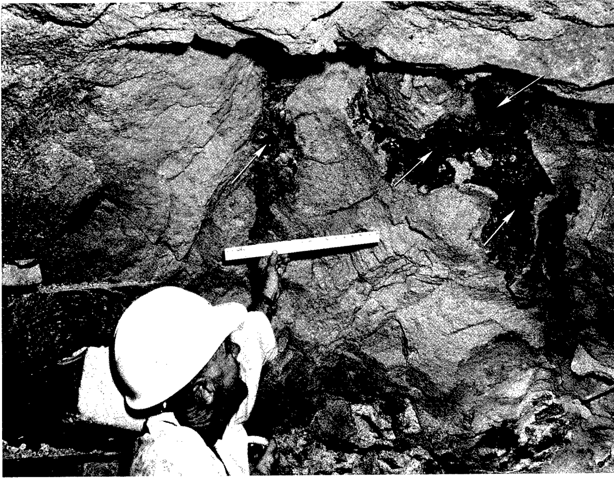
Fig. 35. Wall of a tunnel dug into the vicinity of the cavity of an underground nuclear explosion. The dark areas (arrows) are injected melt that has been quenched in cracks within cold country rock.
