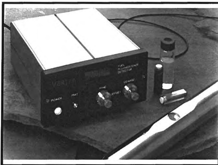
Figure 11. The ARA FFD sensor for the cone penetrometer. The sapphire window through which fluorescence is excited and collected is visible in the side of the probe.
