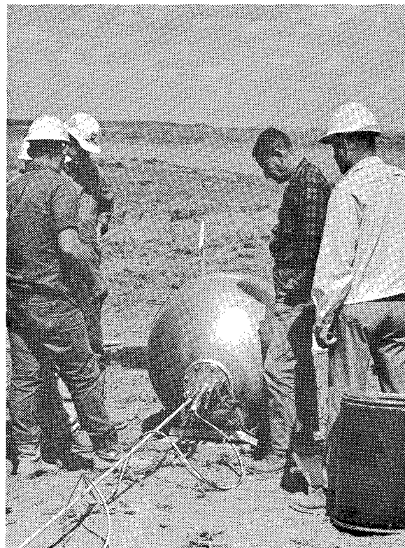
Fig. 6. Charge (1000-lb) for seismic site calibration series and coupled shot of seismic decoupling experiment.
