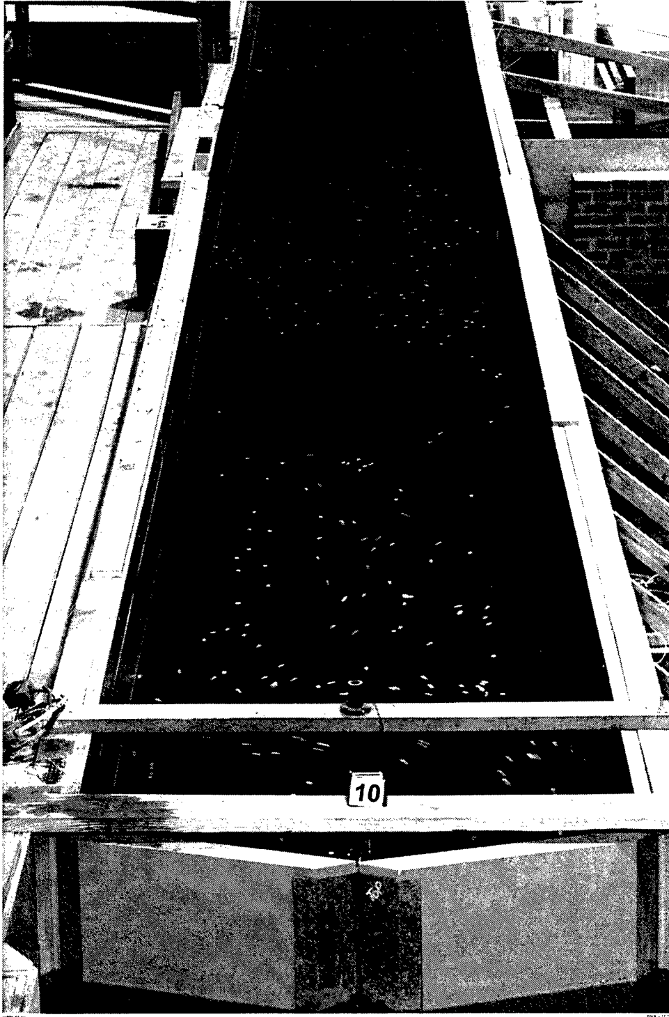
Photo 6. Confetti illustrating surface currents within the lock chamber 10 min after filling started
