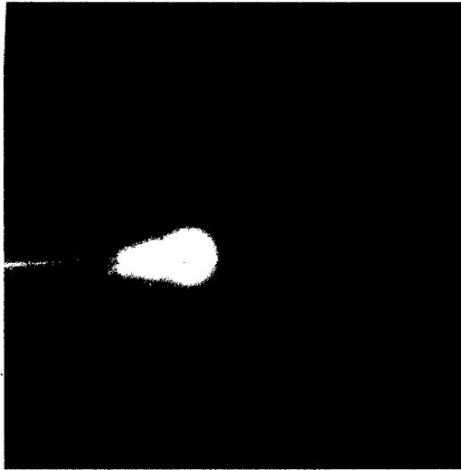
Fig.1. HF discharge near hot electrode in supersonic flow ( M \sim 2 , P_{st} \sim 100 torr).
