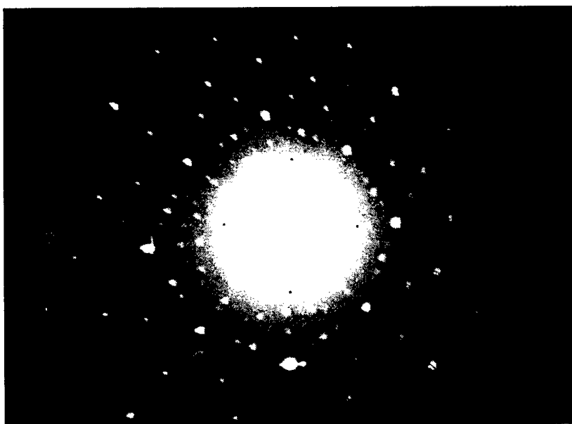
Figure 14. Back-reflection Laue for the W-Ta alloy in the [001] orientation.
