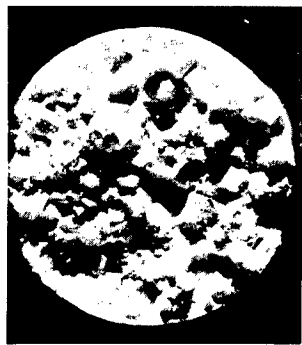
Fig. IVE-1. Uniaxial tension test of LX-04-1 at 68°F; failed normal to stress; illustrates complete molding powder bonding; 3X magnification.
