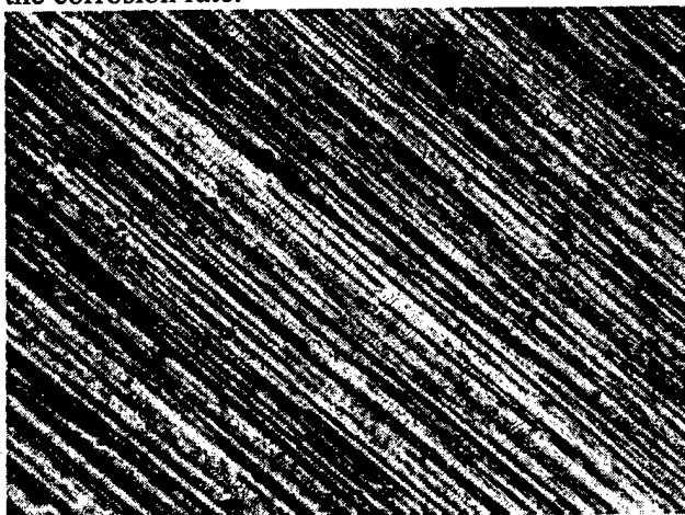
Figure 8 (a). CRS before corrosion (1x 500).
