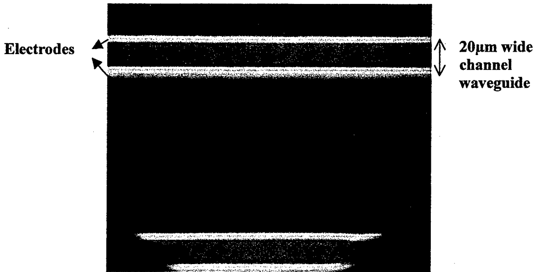
Fig. 3.3.9 The alignment of top electrodes and channel waveguide
