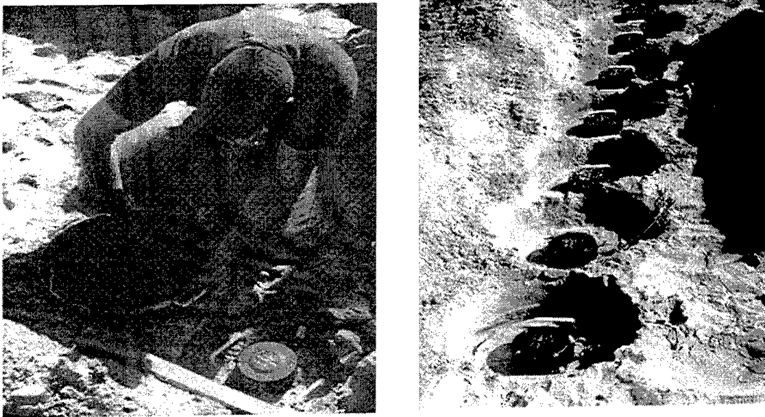
Figure 4.17. Source employment with coffer dam (left) and array prior to burial (right).
