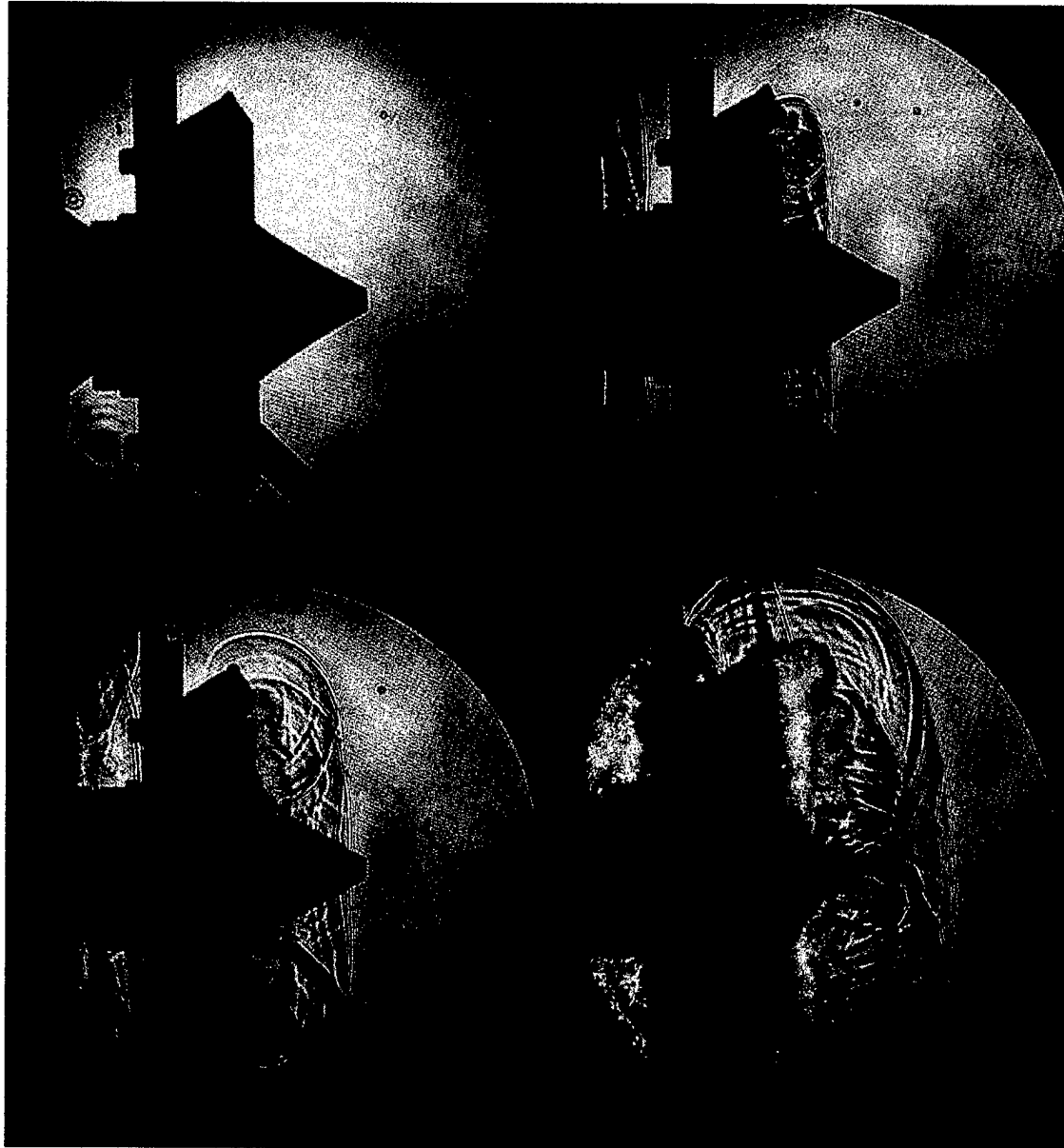
Figure 2. Laser shadow graphs of the shock propagation of an 18 \mu\text{s} carbon dioxide laser pulse impinging on a lightcraft vehicle. The upper left picture shows the vehicle before arrival of a laser pulse. The upper right picture shows the shock after a 30 \mu\text{s} delay, the lower left picture after an 80 \mu\text{s} delay, and the lower right after a 140 \mu\text{s} delay.
