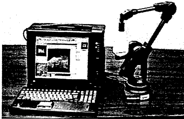
Figure 8. This portable "lunchbox" configuration incorporates a 166 MHz BSI LCD V8 computer 12 , MUSTPAC-2 linear scanner (not shown), MUSTPAC-2 Virtual Ultrasound Probe, and any of several existing ultrasound machines (also not shown).
