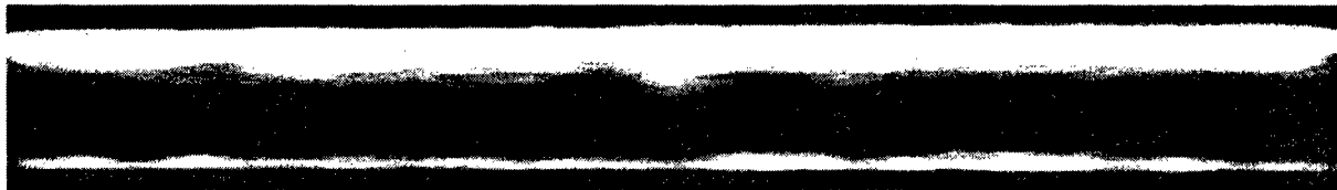
Figure 2: Photograph of a pulsed laser gas discharge with an exposure time of 400 ns during the high voltage pulse
