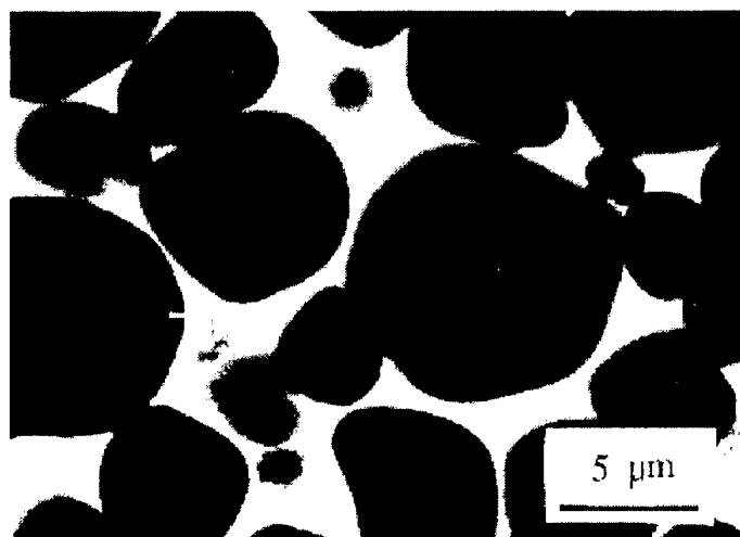
Figure 7.3 Backscattered electron micrograph of stoichiometric TiC-40vol% NiTi. The microstructure, consisting of TiC particles surrounded by a two-phase matrix, is typical of composites synthesized with the anticipation of stoichiometric carbide formation.
