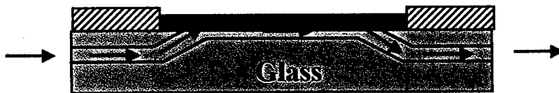
Fig. 1. Cross sectional side view of the heterogeneous electro-optic glass modulator.
