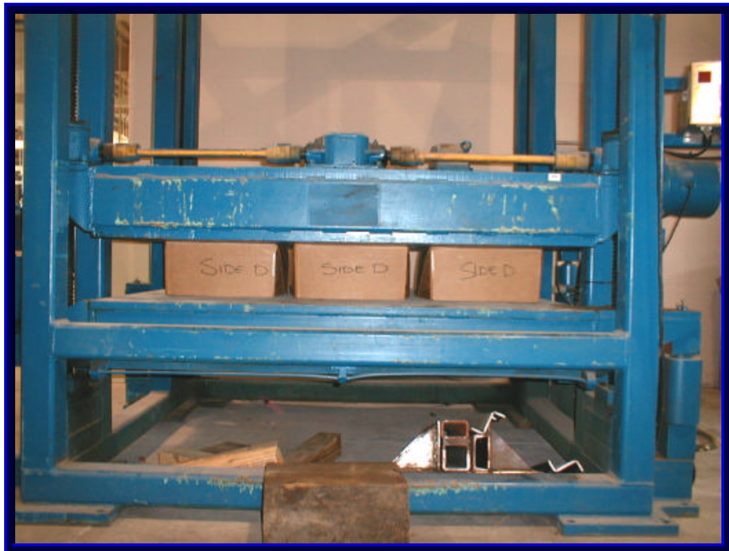
Figure 2. Compression Setup for UN POP Testing
