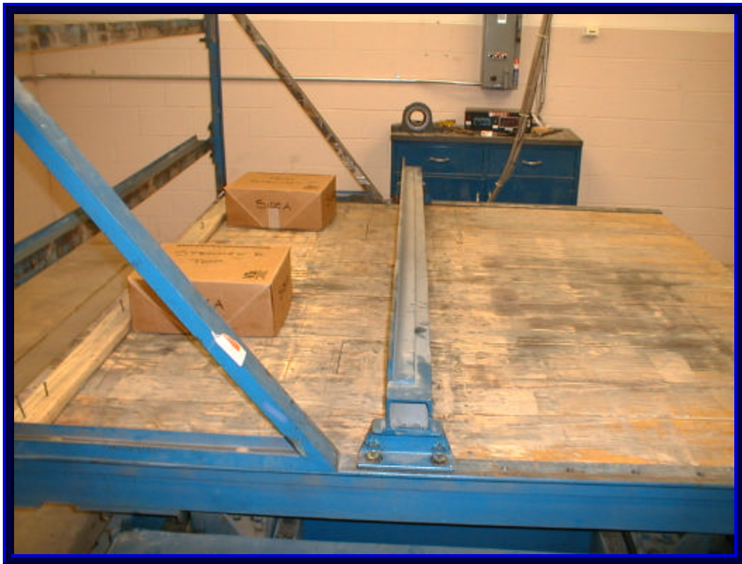
Figure 1. Vibration Test Setup for UN POP Testing
