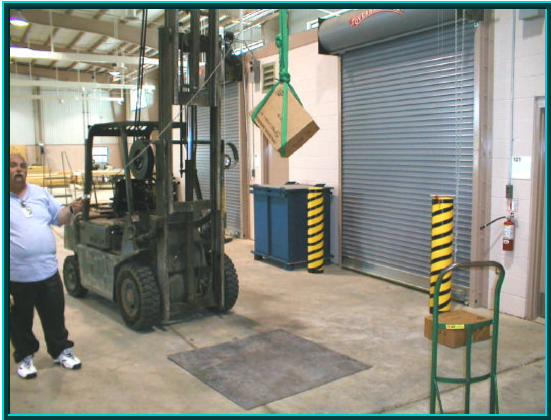
Figure 4. Drop Test Setup for UN POP Testing
